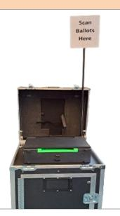
Remove the tamper tapes from the Display Screen and the Printer Access Door and stick them onto the back of the Ballot Scanner Security Record. Place the Ballot Scanner Security Record in the Clear Plastic Envelope.
